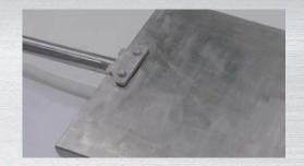
The all new "dove tail" shaft to blade connection utilizes a custom machined locking block that threads onto the stainless steel threaded shaft. This shaft and block combination is then mated into a matched cutout in the heavy duty blade. This combination of perfectly matched CNC machined parts creates a maintenance free shaft to blade connection.
